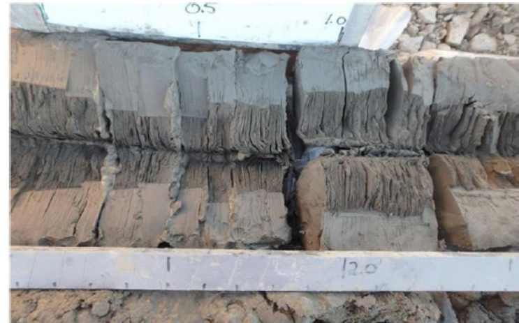
SH14-10 (Middle/Top UGLU Layer) Approximate El. 921.1 m to 919.5 ,m Sub-horizontal varved bedding. Water content = 35.7%; Liquid limit = 60%; Plastic index = 20%; Clay fraction = 58%
